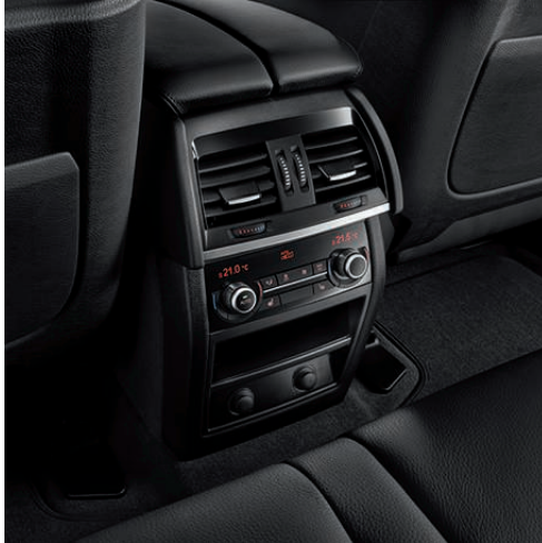
AUTOMATIC AIR CONDITIONING WITH 2- OR 4-ZONE CONTROL. ensures a pleasant interior temperature for greater comfort. You can switch between automatic and manual operation. The automatic air conditioning with 4-zone control shown here also features controls in the rear.
