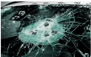
MULTI-LAYERED SAFETY GLASS The BMW X5 Security features safety glass on all windows. The glass is approximately 2cm thick and consists of a glass/synthetic composite capable of withstanding fire from weapons up to a .44 calibre Magnum. A polycarbonate coating on the inside of the glazing prevents glass fragments entering the interior for even greater protection. The multi-layered safety glass looks virtually no different from standard glass.
