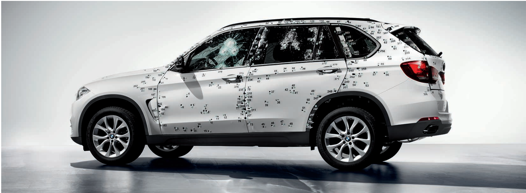
MULTI-LAYERED SAFETY GLASS The BMW X5 Security features safety glass on all windows. The glass is approximately 2cm thick and consists of a glass/synthetic composite capable of withstanding fire from weapons up to a .44 calibre Magnum. A polycarbonate coating on the inside of the glazing prevents glass fragments entering the interior for even greater protection. The multi-layered safety glass looks virtually no different from standard glass.
