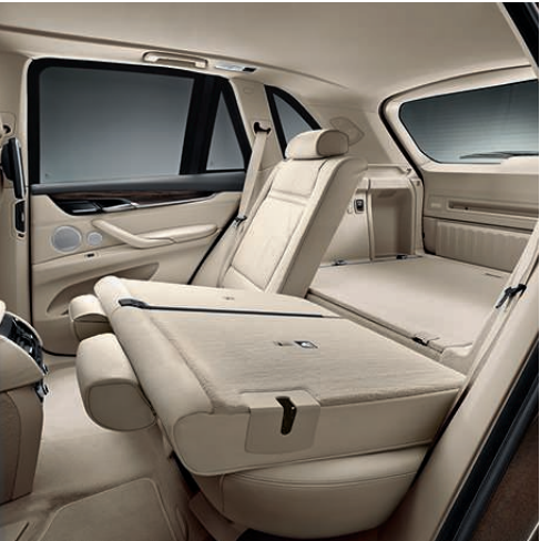
THROUGH-LOADING SYSTEM 40:20:40 features an asymmetrically dividable rear seat backrest for a variety of storage options offered by no other Security Vehicle. Luggage is also optimally protected thanks to the luggage compartment armour and a rear window made of multi-layered safety glass.
